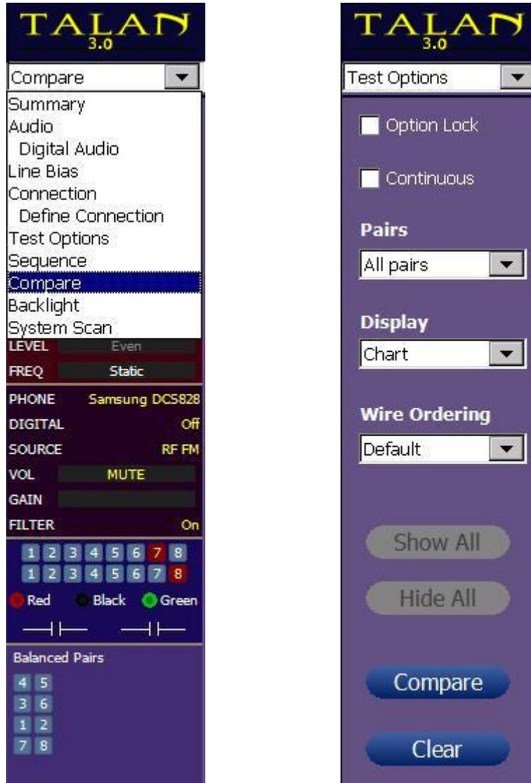
During any test mode, the results are saved in the **A** or **“Live”** position. They can then be compared to a previous test or reference file loaded into the **B** or **“Ref”** position. All TALAN Test functions can be compared using this A/B Comparison mode, however, only an FDR example is provided in this manual as an example.
