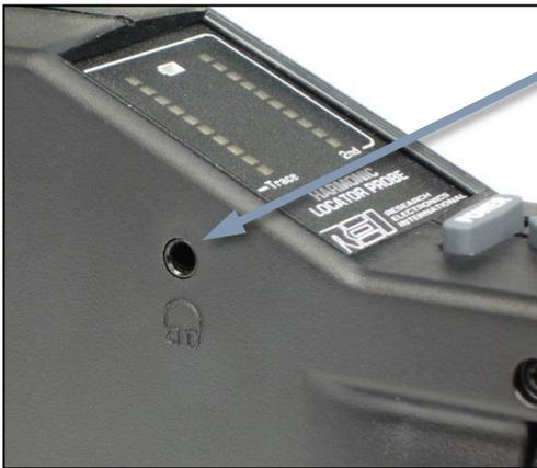
The headphone jack is located on the left side of the unit. It accepts a standard mono 3.5 mm plug. It is recommended that headphones be used to be non-alerting, if required. Using headphones instead of the speaker can also extend battery life.
