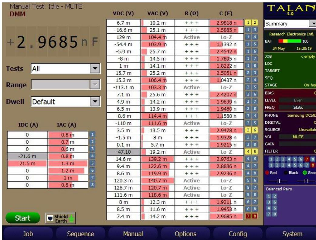
There may be situations where signal conditions are such that a given test does not remain on the pairs or wire long enough to be able to give a reliable reading. For these instances, the user can change the **Dwell** time selection from **Default** to **Extended**.
