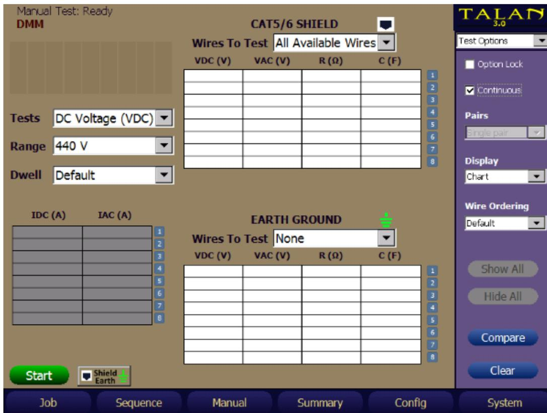
The **Shield** and **EarthGround** testing interfaces are shown. The normal **Test Options** selection for **Pairs** is not functional for **Shield** or **EarthGround** testing. However, there is an individual selection for each now. This allows the testing event to be customized. The **Wires To Test** can be customized through the drop down menu item individually for the **Shield** or the **EarthGround** to **All Available Wires**, **Selected Wire**, or **None**.
