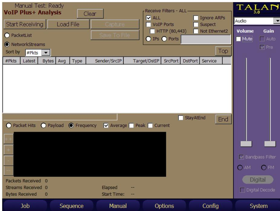
**Start Receiving** performs analysis of actual network traffic happening right now. **Load File** performs analysis of data that has already been collected in a file. The file types accepted are standard **PCAP** files.
