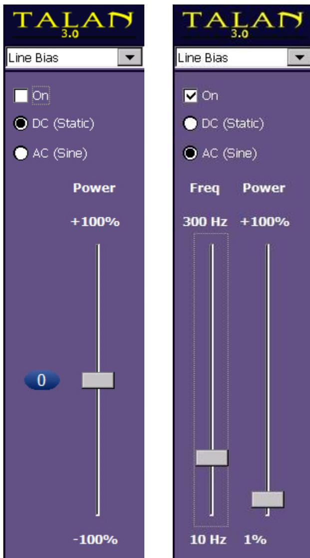
**It is highly recommended that the rotary dial be used to adjust the power level of the Line bias function. The rotary dial provides a much finer control, while the stylus may provide quick, large, jumps in voltage. You should be careful not to put too much voltage on a line.**
