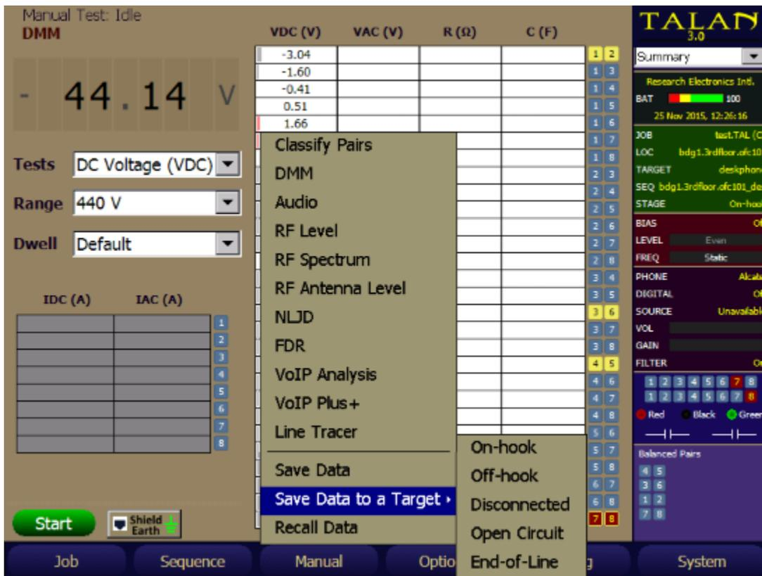
Select the stage for this test, e.g. **On-Hook**, **Off-Hook**, **Disconnected**, etc. for the appropriate test type and physical setup. Note: This list of stages varies depending upon the test type (DMM, Audio, etc.) and the stage selected.
