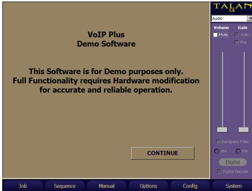
Selecting **Continue** permits the Control Interface to be displayed, but it is non-functional in that it will not receive packets nor load and run files. The figure below shows the fully functional TALAN VoIP Plus+ Control interface:.
