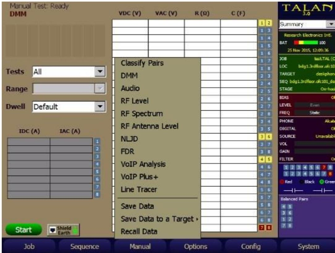
The manual test controls for each function are very similar. For each test, once the test pairs have been defined (single, balanced or all) under the Test Options dashboard, and any other test parameters have been specified, the test is started by pressing the **START/STOP** button or tapping Start on the screen.
