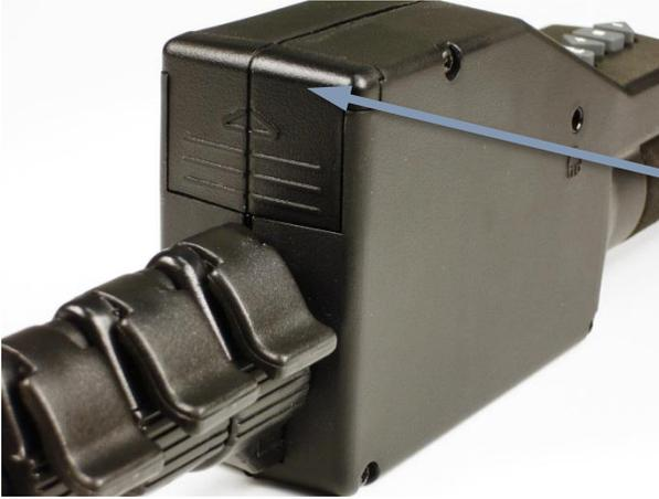
The power source is a 9 V alkaline battery. There is a sliding door that is used to retain the battery. Insert the battery in the correct orientation as indicated by the label inside the compartment.
