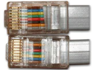
The TALAN can be used “in-line” with a phone system using the TALAN’s two modular jacks which are identified as LINE and PHONE. The modular jacks on the TALAN are wired straight through to allow for most common telephone systems without the use of a special crossover or special test adapter cable. Pin 1 on the LINE jack corresponds to Pin 1 on the PHONE jack and so on.
