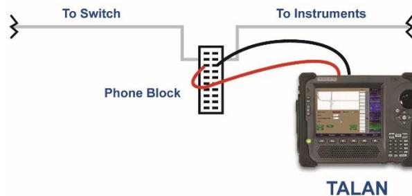
It is important to understand that prior to interrupting the phone line you should first verify that there is no audio passing down the line. Therefore, regardless of where you test the line, you should first use the banana plugs, connect to the main audio pair and test for audio. This is often easier at an intermediate block. Then, it is recommended that the user start testing at the phone set. For the remainder of this document, it is assumed that the testing is performed at the phone set.
