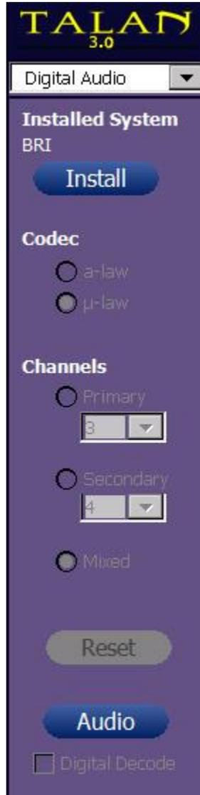
The Codec indicates the type of modulation that is used.  $\mu$ -law is used primarily in North America and Japan while a-law is prominent in the rest of the world.
