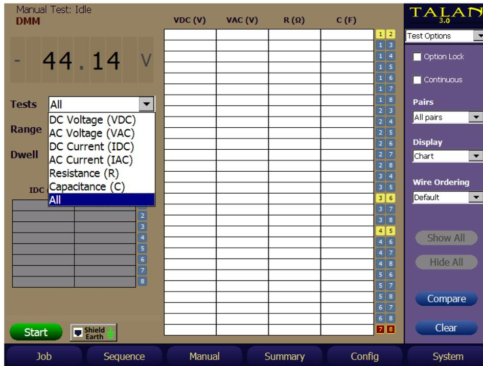
Then, select which tests to measure as shown above. It should be noted that to prevent a non-practical test there are automatic conditions for performing some of the tests (for example, you cannot measure capacitance on a line that is terminated or powered).
