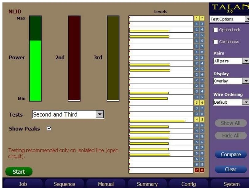
To determine the proper pair with the tap, the transmit power is manually decreased until only the true pair shows an NLJD response.
