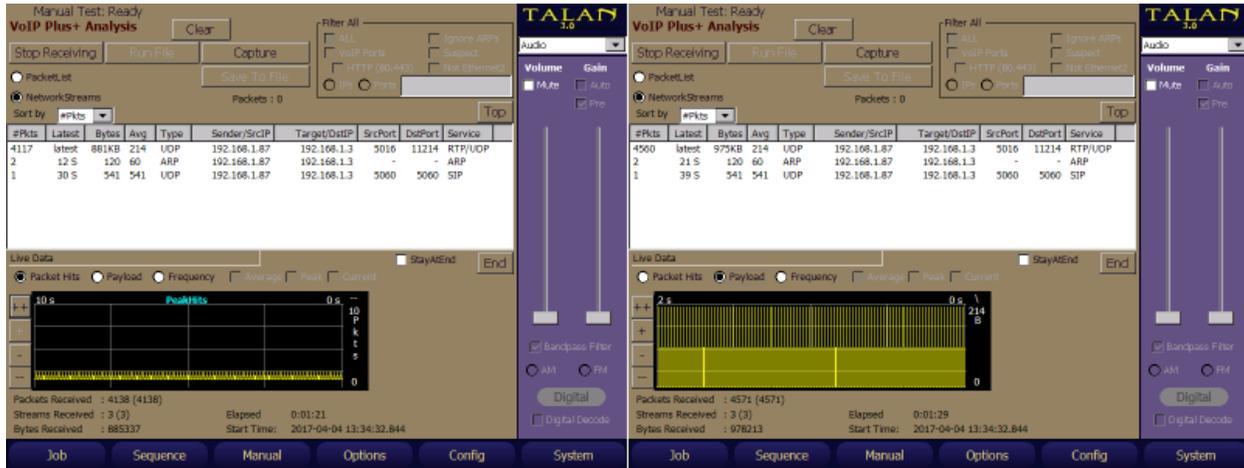
Look at the original VoIP Plus+ Control interface. It shows the main two analysis methods of **Start Receiving** and **Load File**.
