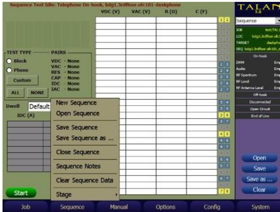
Within the test Sequence, different stages will be defined as previously described and specific tests will be available under these test stages as indicated by the example menu structure below.
