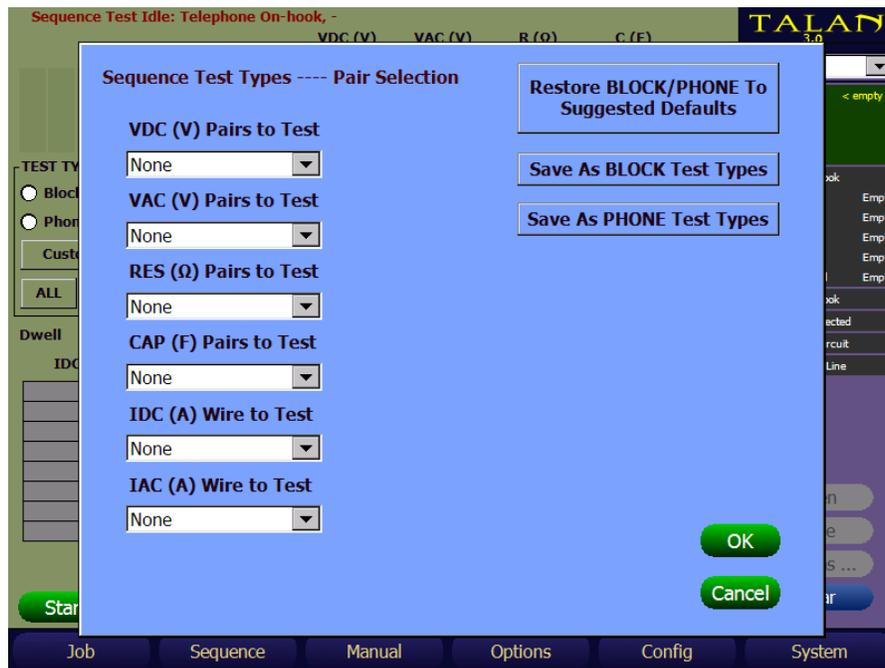
Using the above shown display, each individual **TEST TYPE** can be modified to the desired setting.
