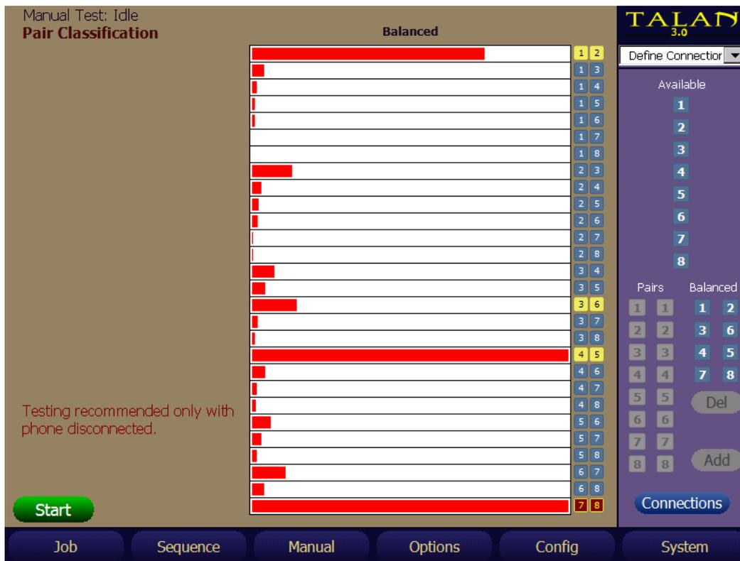
After reviewing the balanced line data, you should manually define the combinations of balanced pairs by selecting them in the Define Connections dashboard. Tap the connector numbers that make up the pair and select Add to define the pair as a balanced pair. Once the balanced pairs have been defined, all other test screens will display the balanced pairs with a yellow background.
