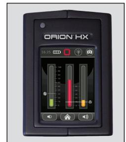
Tx and Rx graph displays power, 2nd and 3rd harmonic levels and touch screen trip and power level adjustments.
