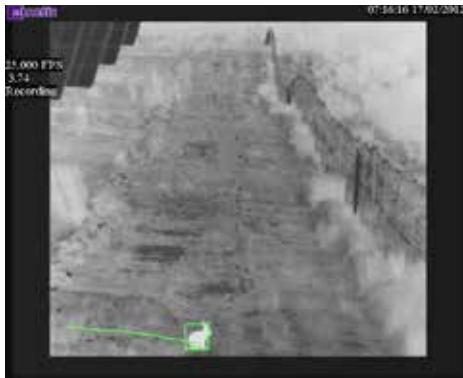
Animals are considered as authorized intruders and will not trigger the alarm.
