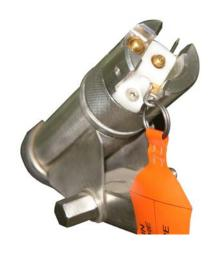
Breech with safety pin. EDS-11 breach assembly has been recently improved to incorporate a safety pin. This enables a bomb technician to set up the disrupter with firing lines at the incident control point. It ensures safe deployment of the disrupter and spending minimum time at the IED. The terminals are made heavy duty springs for contacts with cable reels.
