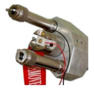
EAD-20 breech has a safety pin to keep the terminals short and cartridge is connected just when it has been deployed. This enables a bomb technician to set up the disruptor at the incident control point and spending minimum time at IED
