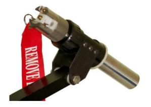
Breech with safety pin. Disruptor breech has a safety pin to keep the terminals short and cartridge is connected just when it has been deployed. This enables a bomb technician to set up the disruptor at the incident control point and spending minimum time at IED.
