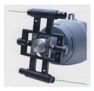
Different sets of jaws are provided to hold firmly onto different shapes of fuzes. It can generate torque in both clockwise and anti-clockwise directions. The electrical cartridges can be initiated using an Electronic exploder or a wireless remote detonation system.
