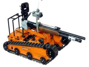
Actuation Mechanism, Laser Aiming, Camera and LED light. In EOD or IEDD operations remote controlled shot guns are used to gain access or shoot an area of interest. The gun used for the system is a multi-shot and semi-automatic. The gun has the capability to fire five shots. To install the gun on any robot the complete assembly is fitted to the Arm of the robot and connected to the local firing terminals.
